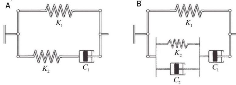
**Figure 1.** A) Standard Linear Solid Model (SLS) and B) the Four Element Model (FEM)
